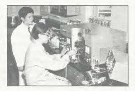
An atomic absorption spectrophotometer was used to analyze samples for calcium and other minerals.
